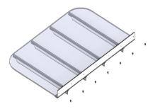
**STEP 3:** Align slots in back panel with holes in back bar and secure with screws from STEP 1.
