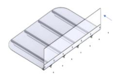
**Step 2:** Align the left side "L" and right side "R" of back panel with the left side "L" and right side "R" of well cover.
