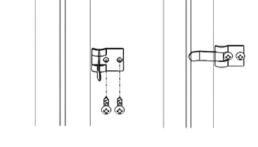
**Note:** If assembling quick-release clips to concrete or brick, use a 3/16" masonry bit to drill each clip hole to a 1%" depth. Use a hammer to insert masonry anchors provided and then screw the clips into the anchors in the concrete/brick.
