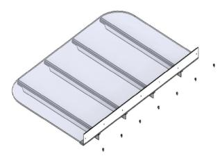
**Step 2:** Align the left side "L" and right side "R" of back panel with the left side "L" and right side "R" of well cover.
