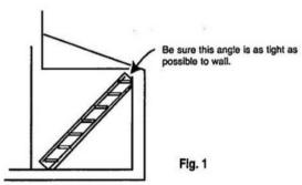
STEP 3 CUT STEPS from 2" x 10" lumber. The cut size will be 2" less than the width between the walls supporting the STEELWAY STAIR STRINGER.
